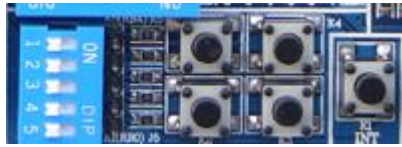
Figure 4-30 Independent Key and External Interrupt Module
