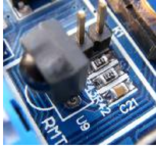
Figure 4-20 Remote decoding module
