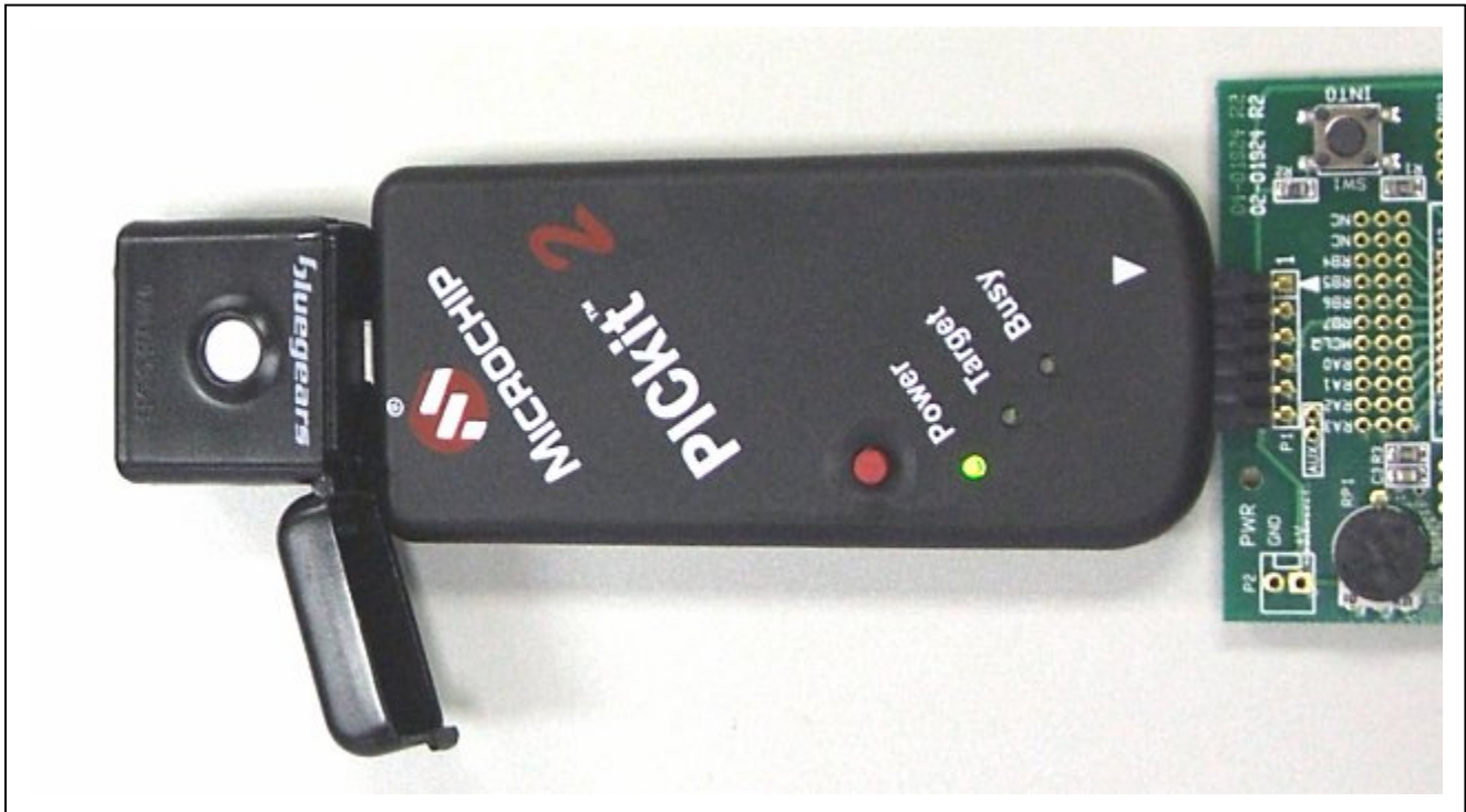
FIGURE 2-2: B-MOBILE POWERING PICKIT 2 UNIT FOR PROGRAMMER-TO-GO OPERATION
