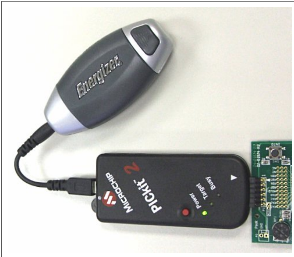
FIGURE 2-4: ENERGI TO GO POWERING PICKIT 2 PROGRAMMER-TO-GO
